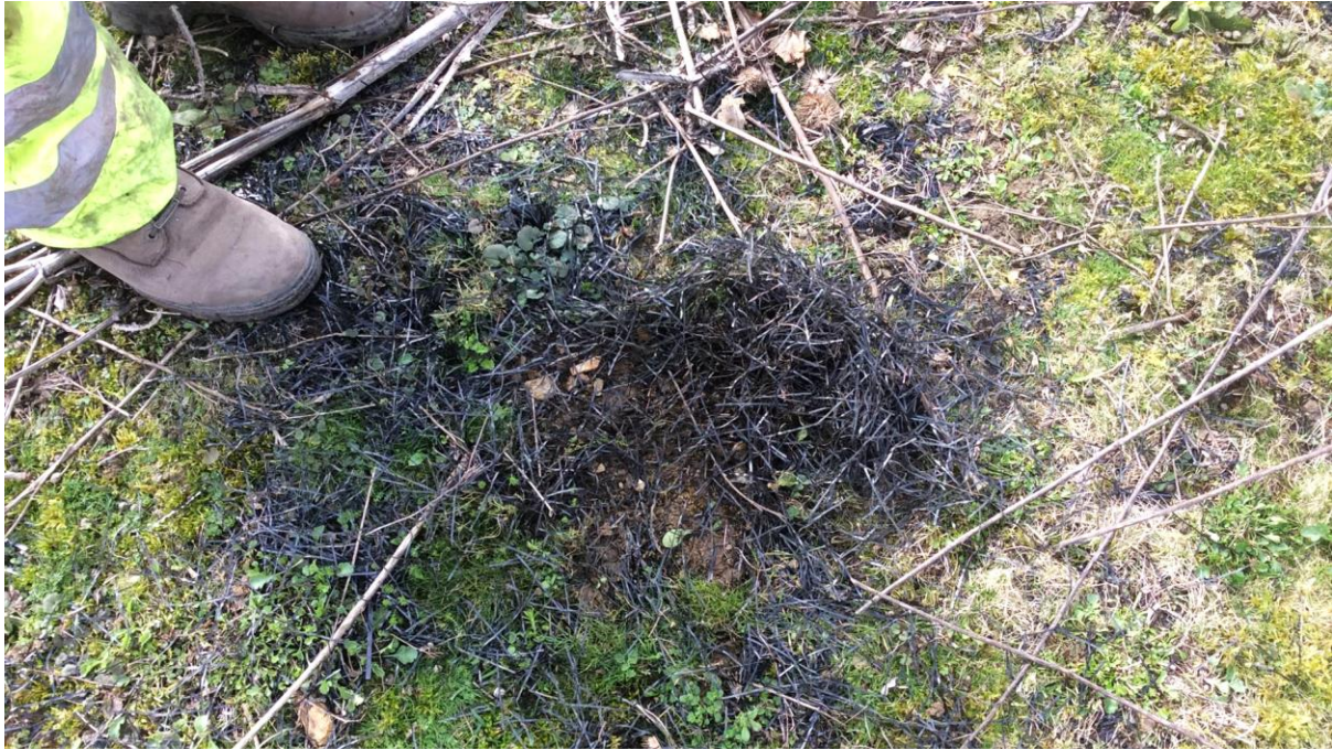
Figure 7: Fibres present on the ground surface and to a lesser degree in the exposed made ground
